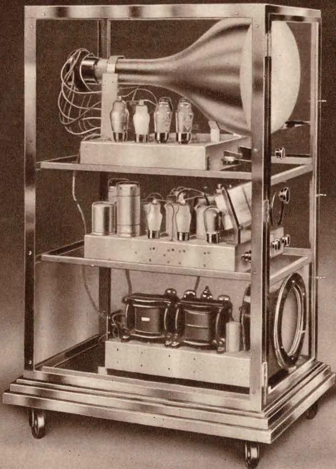
The "three deck" chassis of the Cossor Television Receiver. Above the upper deck is the Cossor Cathode Ray Tube. The middle section houses the Radio receiver, while below is the power pack and moving coil speaker.
