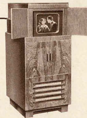
As used for Receiving Television. When not in use the doors are closed to protect the end of the cathode ray tube. The tuning dial and controls are protected by the lower doors.
